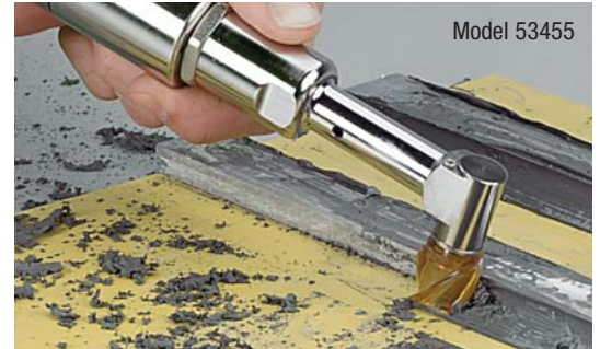
Right: 53455 Drill powers optional 3M "SR Cutter" accessory for fast, aggressive removal of seam sealant.
